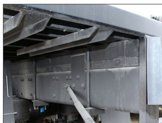
Structural C-channel Long Sills (ILO I-beam)
